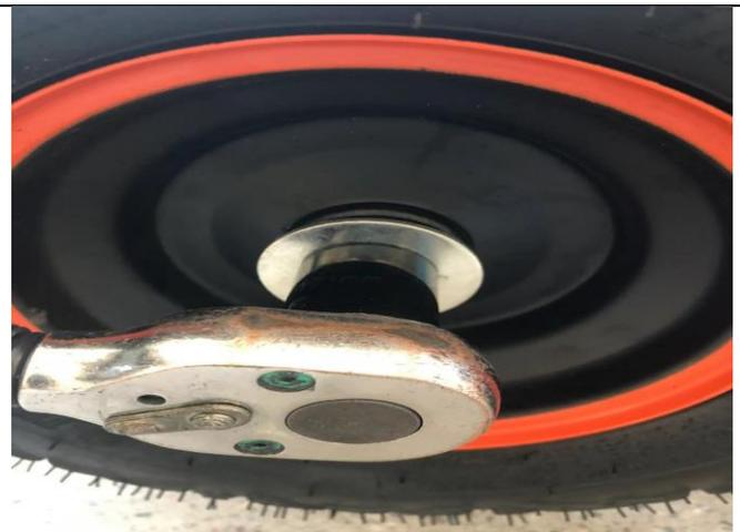
8. Align the rear wheel with the splines (I) and push on the rear axle, with the air nozzle cap facing outward, Use tool ①⑥ to lock the nut (F) and washer (B), then insert the cotter pin (G), keep the bending angle greater than 180°
