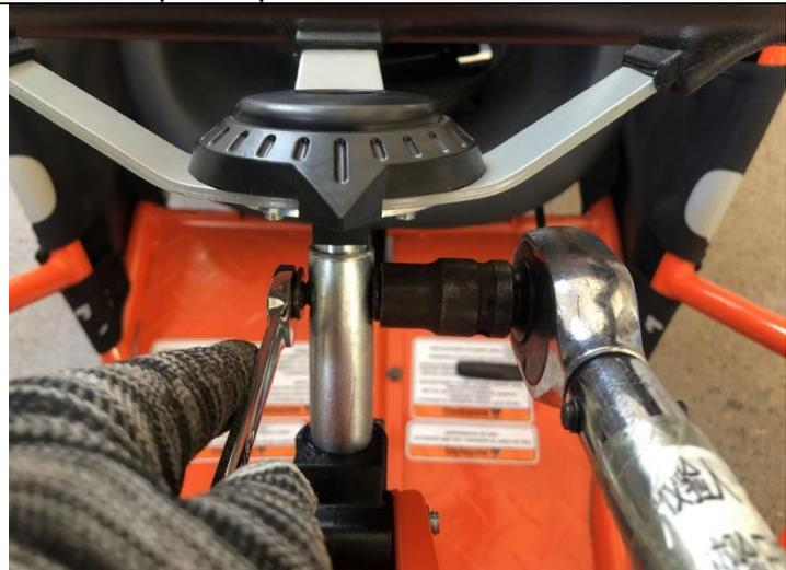
10. Put the steering wheel with the steering column, use tool ①⑤③ to lock (D)
