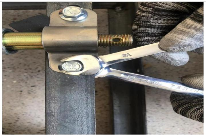
6. Use tool ②③ to remove the screws mousing on the rear axle, put the vehicle on the stand for easy installation of other accessories.
