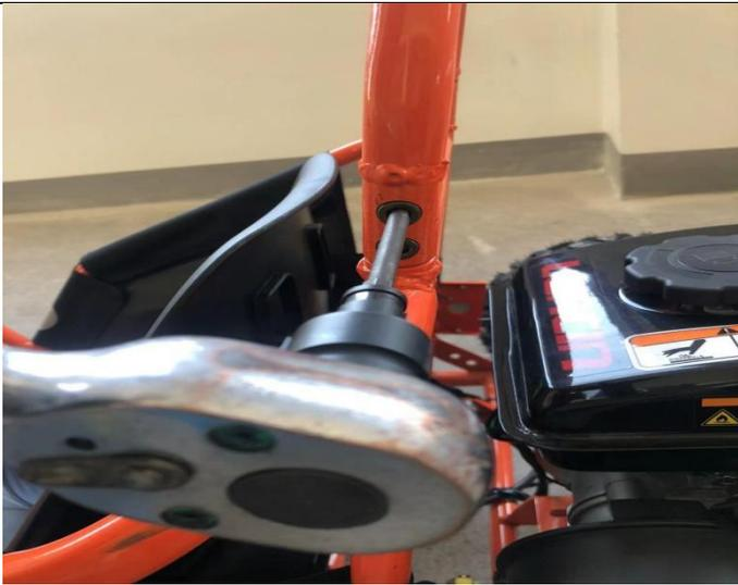
11. Put the rear guard to the fram, use tool ①④ to tighten (C).
