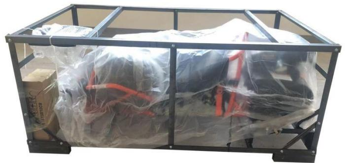
3. Take out the parts attached on the vehicle and the packaging iron frame, remove the iron frame screws, wait for subsequent installation.
