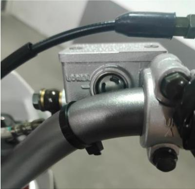
K2 model use hydraulic disc brakes, and the brake fluid level of the disc brakes can be checked through the observation hole.
