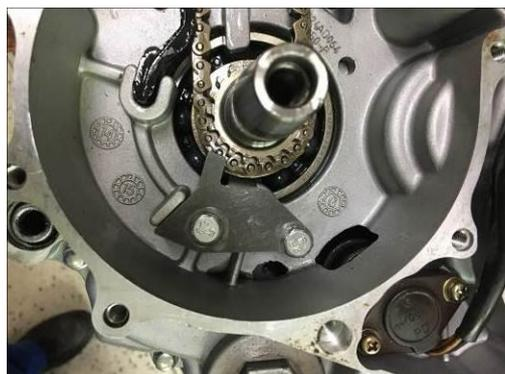
1. Place the left crankcase of the engine upwards;
