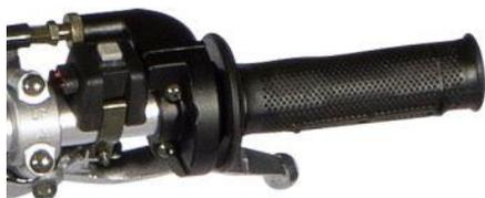
The throttle knob is located on the right side of the handlebar and is controlled by turning with the right hand. When the handle is turned counterclockwise, increase the throttle, release the handle and return it to the position.
