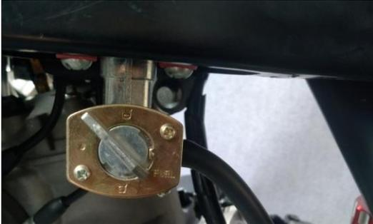
The K2 carburetor version adjusts the fuel supply through the fuel tank switch, which is located at the bottom of the left side of the fuel tank. By rotating the switch, you can control whether the fuel enters the carburetor, so as to achieve the control effect.
