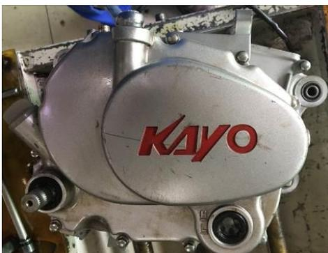
1. Drain the engine oil first (remove the oil filter cover on the left, take out the spring and oil filter combination, wait for the oil in the box to run out, and then remove the oil filter cover, pay attention to the oil filter Whether the O-ring of the cover is damaged;
