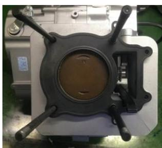
1. Remove the cylinder head gasket combination;
