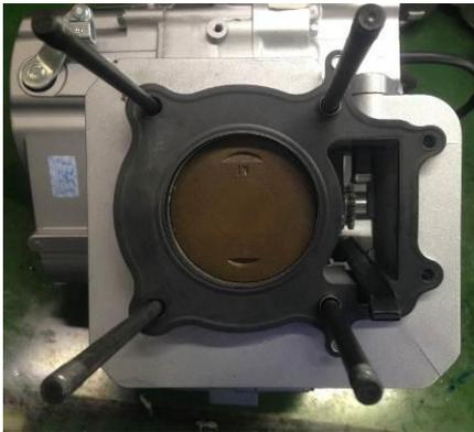
1. Install cylinder block positioning pins and new cylinder block gaskets;
