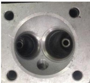
Completely remove the carbon deposits in the combustion chamber, apply a thin layer of red stamping oil evenly on the valve seat, place the valve on the valve seat and knock the valve lightly without rotating, and then pull out the valve. If the contact marks on the valve working surface are discontinuous, the valve seat should be polished and repaired.
