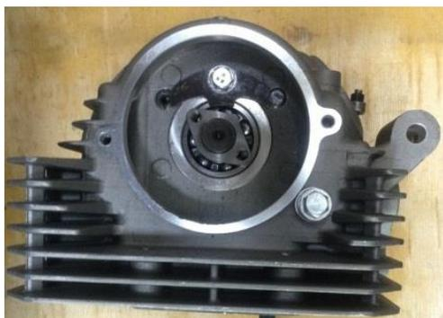
1. Remove the camshaft limit bolt;
