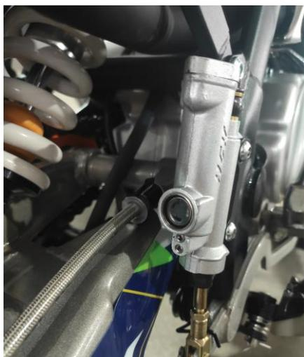
Observe through the liquid level hole to check the level of brake fluid. The liquid level should exceed half of the observation hole, that is, the liquid level should be higher than "LOWER". If the brake fluid is insufficient, it should be added immediately.
