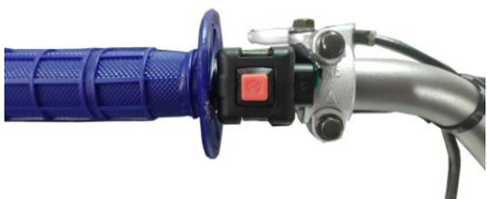
The engine's stop switch is located on the left side of the handlebar near the grip. It is a square red button. Long press it to turn off the engine.
