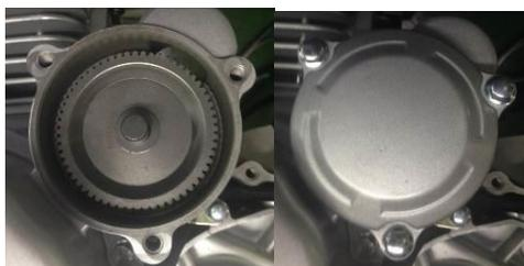
1. Install the double gear washer on the end face of the double gear;
