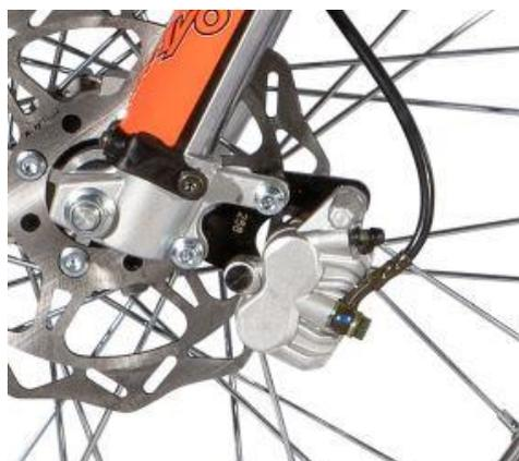
The front brake adopts a floating caliper disc brake, which is installed on the lower end of the left front shock and fixed by 2 bolts.
