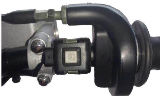
The vehicle start button is located on the right side of the handlebar, close to the position of the throttle knob. It is a square gray button. Long press it to start the motorcycle engine. In addition to the start button, the vehicle can also be started by stepping on the start lever.
