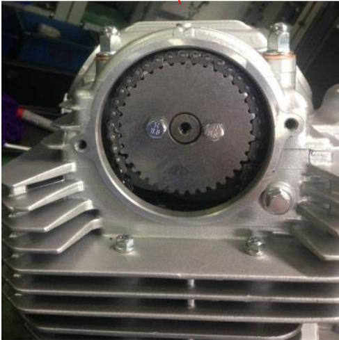
1. Replace the new cylinder head gasket combination, install the positioning pin, and assemble the cylinder head;
