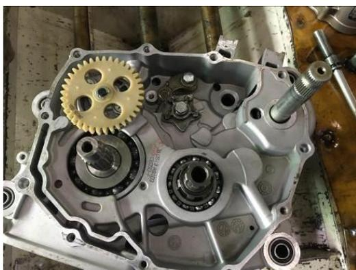
1. Remove the oil pump fastening screws;
