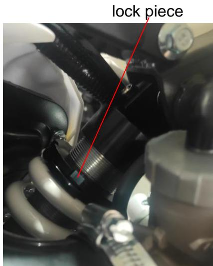
The spring preload of the rear shock absorber can be controlled by adjusting the lock piece. Adjust the lock piece to move down, the spring preload increases; Adjust the lock piece to move up, the spring preload is reduced.
