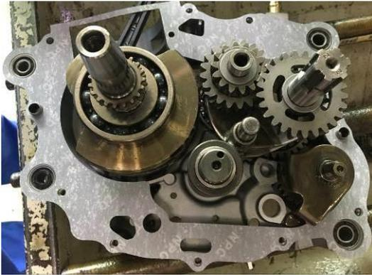
1. Take out the crankshaft assembly from the box;
