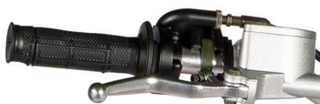
The front disc brake is controlled by the brake lever. Which located at the right end of the handlebar, and operated by the right hand.
