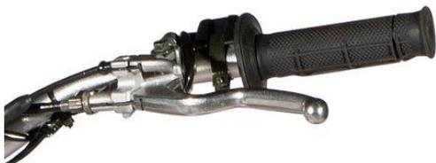
The clutch is controlled by the clutch lever, which located at the left end of the handlebar, and operated by the left hand.
