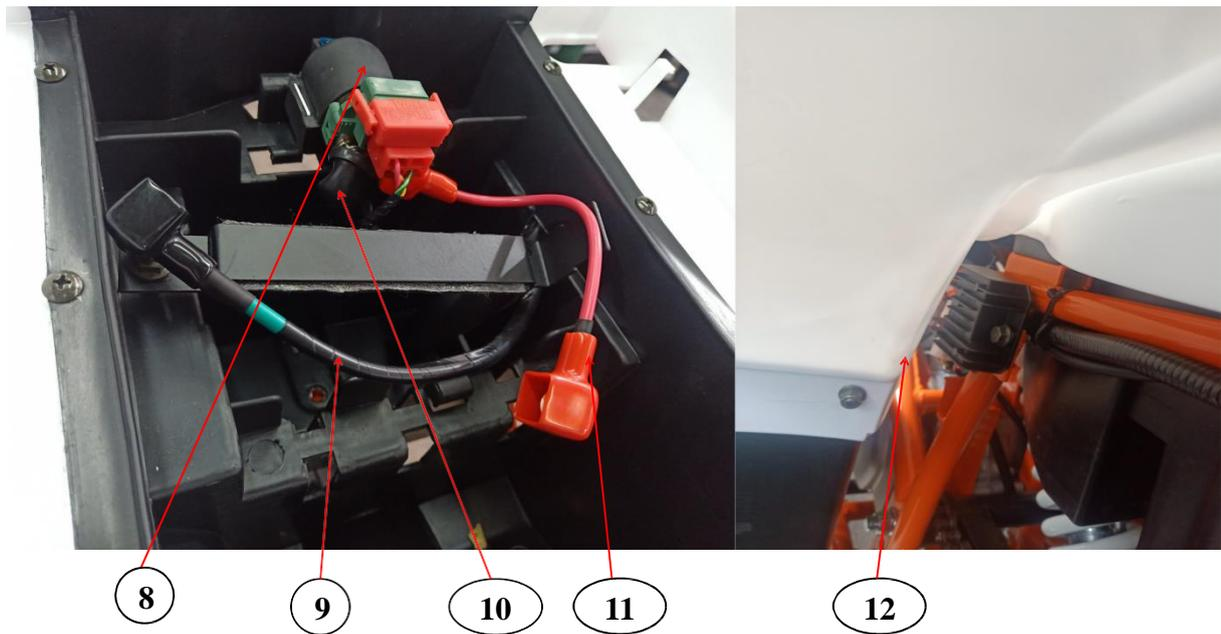
8. Relay 9. Battery negative wire 10. Starting motor wire 11. Battery positive wire 12. Voltage stabilizer rectifier
