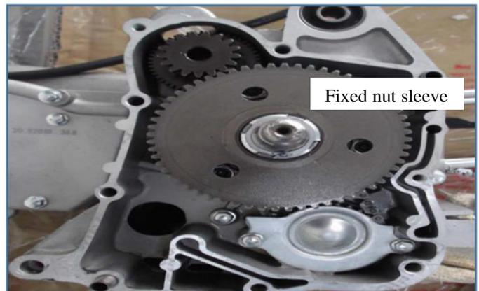
Remove the starting driven gear.
