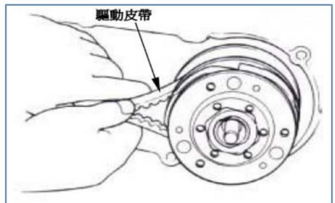
Squeeze the drive belt into the groove of the drive pulley as shown in the figure to loosen it, and then take out the belt and clutch at the same time. Remove
