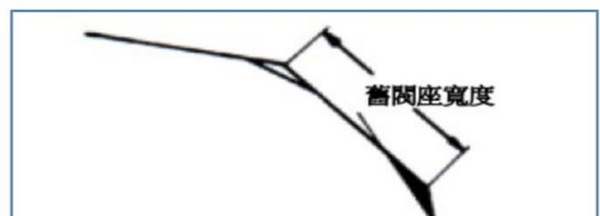
Use a 45° cutter to grind the seat surface to the specified width.
