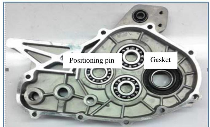
Coat the lip of oil seal of drive shaft, wheel output shaft and gear shaft with butter, install
