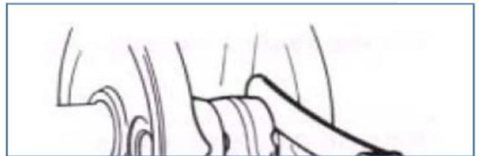
Measure the radial clearance of the big end of the connecting rod in the vertical direction of the crankshaft.
