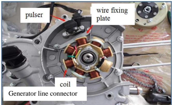
Remove the six bolts of the pulsator, generator coil and wire fixing piece, and take out the alternator coil assembly.
