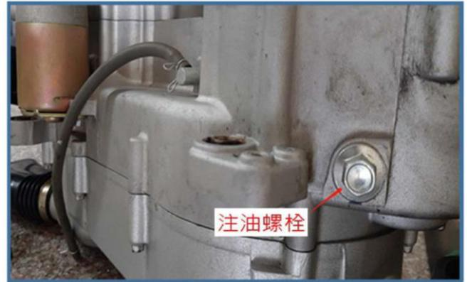
Remove the gear oil injection port bolt, place a measuring cup under the drain bolt, remove the gear oil drain bolt, introduce the gear oil into the measuring cup, and check whether the gear box oil meets the standard value. If the amount of oil is too low, add gear oil.
