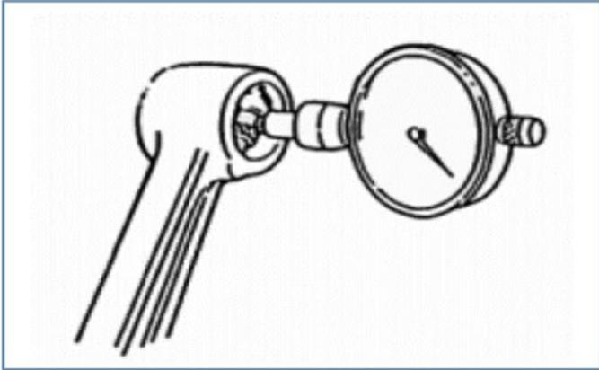
Measure the inner diameter of the piston pin hole.
