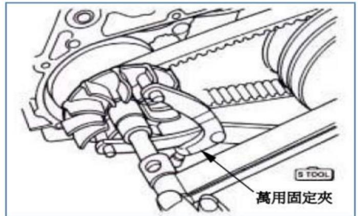
Use the universal fixing clip to fix the clutch cover, and remove the nut and clutch cover.
