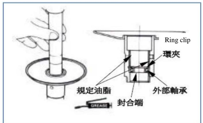
Remove the retaining ring of the outer bearing, and then push the bearing out towards the inner bearing. Push the new bearing into position, and its sealed end should face outward. Apply the specified grease, and install the G-3 grease on the ring clamp to fix the bearing.
