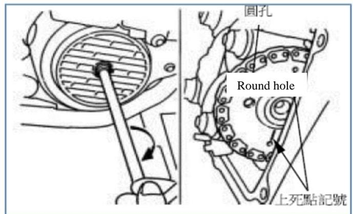
Remove the nut and washer of the camshaft fixing seat.
