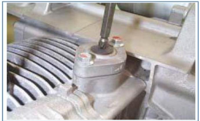
Rotate the flywheel clockwise with a T-shaped wrench to align the "T" mark on the flywheel with the crankcase mark. The upward position of the round hole on the cam gear is the top dead center of compression.
