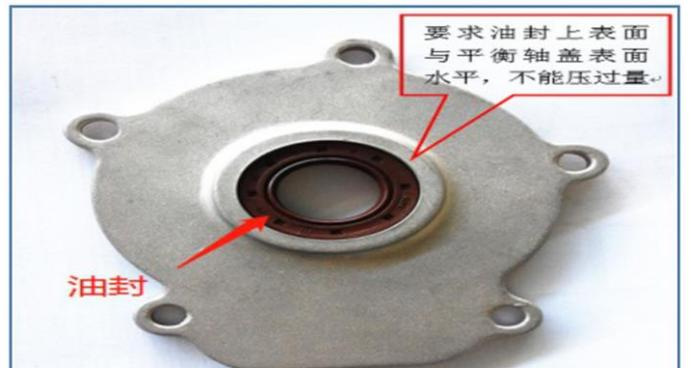
Remove the balance cover oil seal
