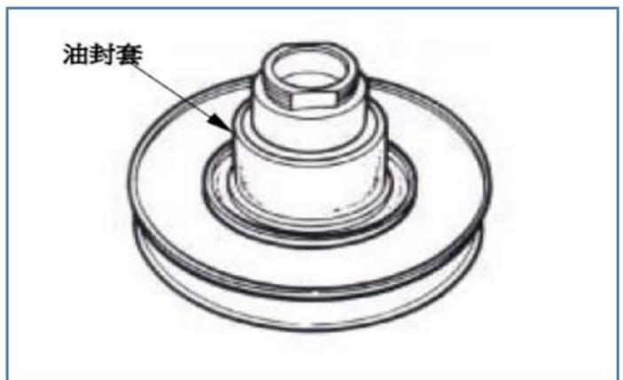
Install the oil seal sleeve.
