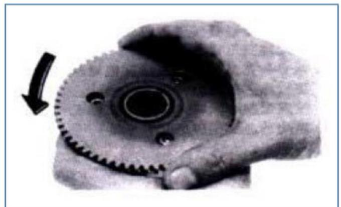
Fix the starting clutch and rotate the starting driven gear.
