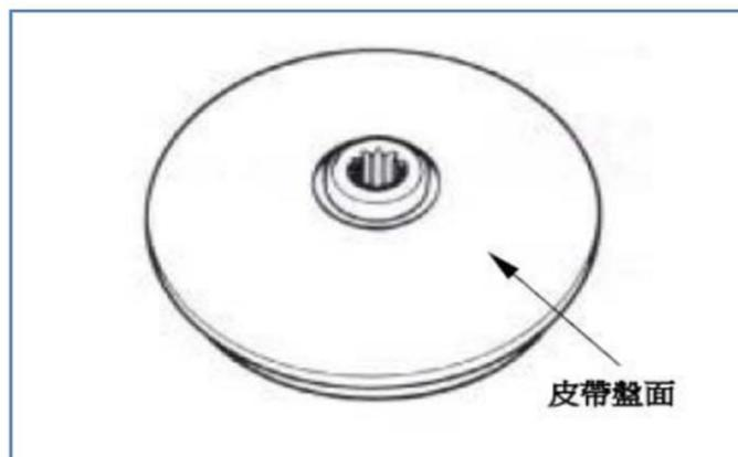
Install the sliding drive plate assembly on the crankshaft.
