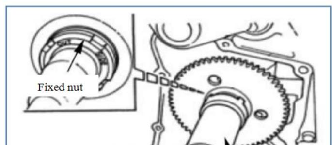
Apply engine oil to the threads of the fixed nut.
