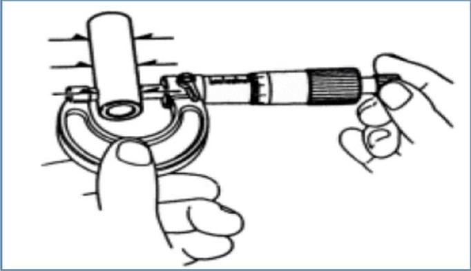
Measure the inner diameter of the small end of the connecting rod.
