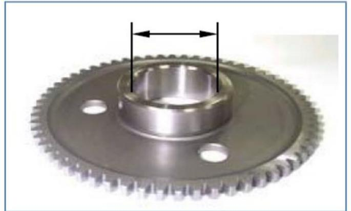
Check whether the starting idler gear and shaft are worn or damaged.
