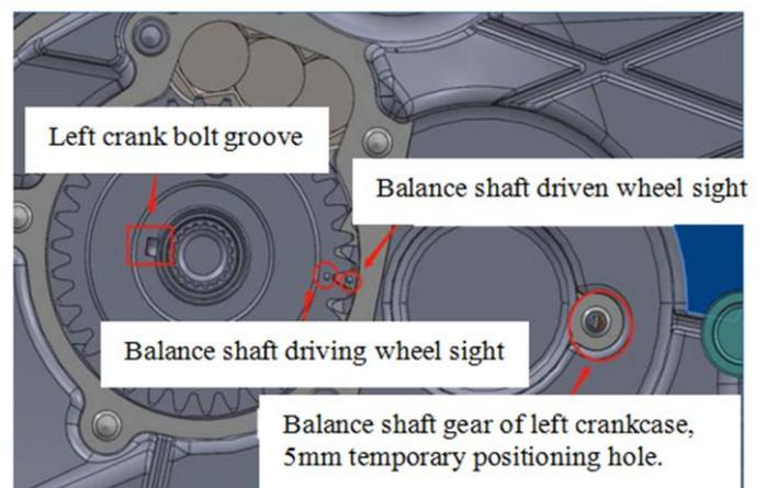
When installing the balance shaft driving gear, ensure that the balance shaft driven gear is temporarily positioned, use the 5mm positioning pin to insert into the gear hole of the left crankcase balance shaft for temporary positioning. Using the front sight on the driven gear of the balance shaft as a reference, and install the star on the driving gear of the balance shaft and the bolt groove on the left crankcase.
