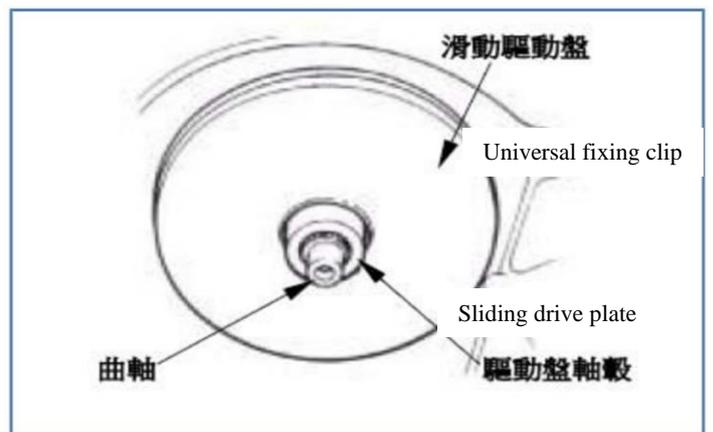
Remove the inclined plate.
