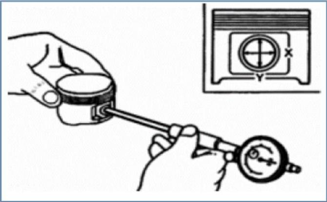
Calculate the clearance between the piston tip and the piston tip hole.
