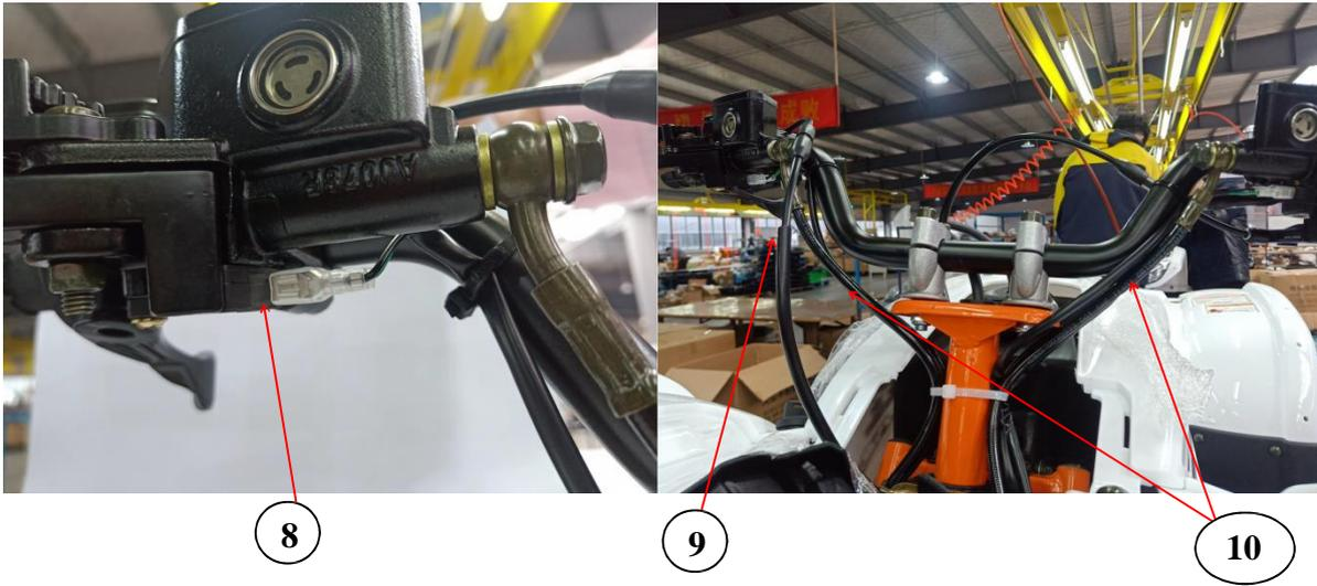
8. Brake sensor (one for left and right) 9. Throttle cable 10. Brake oil pipe
