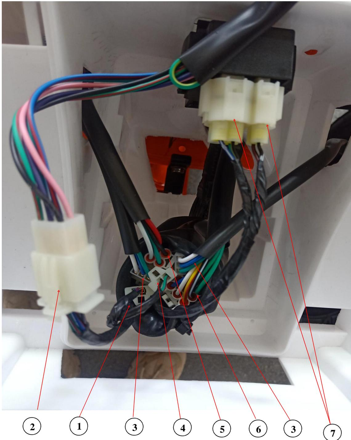
1. Gear display connector 2. Gear indication connector 3. Headlamp connector 4. Spare neutral display connector 5. Electric door lock switch connector 6. Left handle multi-function switch connector 7. Igniter connector
