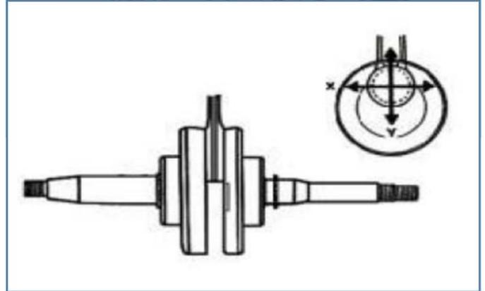
Place the crankshaft on the V-groove block, and measure the crankshaft yaw at the two points shown in the figure with a dial gauge.
