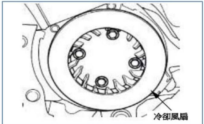
Remove the cooling fan (bolt X4)
