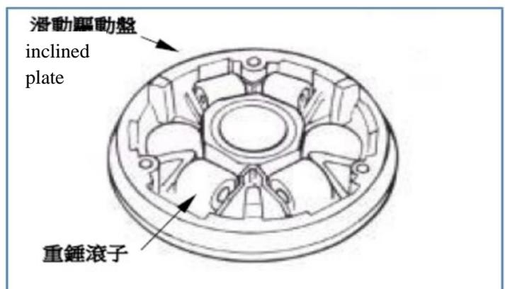
Remove the hammer roller from the sliding
