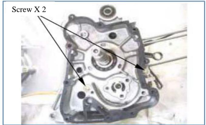
Remove 5 balance shaft cover bolts from the left crankcase, and remove and pull
