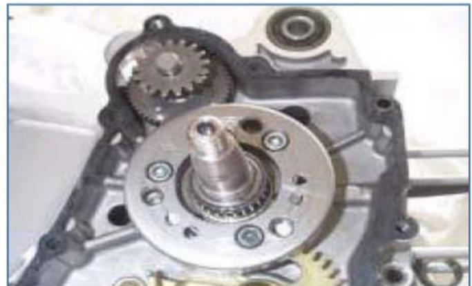
Remove the starting clutch, starting idler and shaft.
