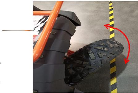
Remove the front wheel when there is shaking, and check the wheel hub
