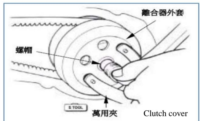
Fix the clutch jacket with a universal fixing clip and tighten the nut to the specified torque value.
