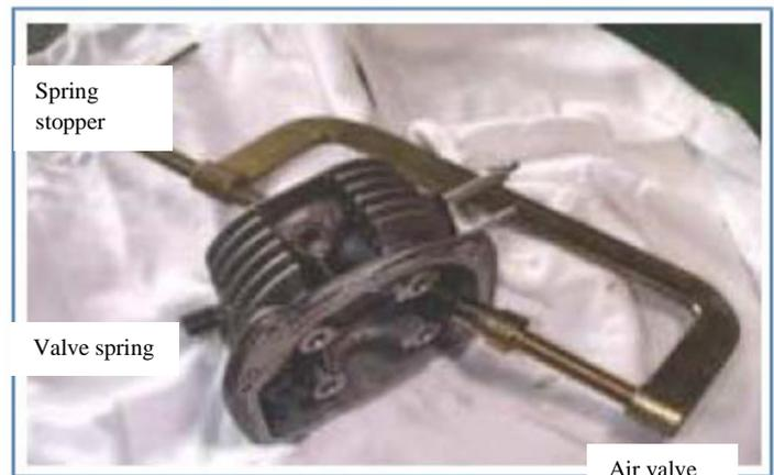
Use a valve compressor to depress the valve spring.
