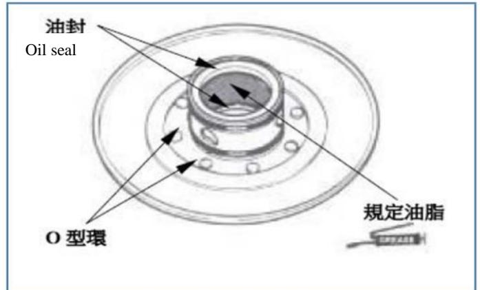
Install the sliding drive plate on the drive belt plate.
