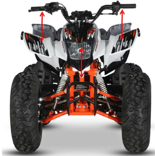
Place the car in a horizontal position and slowly turn the direction handle to the left and right to confirm whether it can turn smoothly and flexibly. If there is obstruction in some places, check whether the main cable assembly and cables interfere. If the end Position of the steering pull rod is not observed, confirm whether there is interference and whether the steering bearing is damaged.
