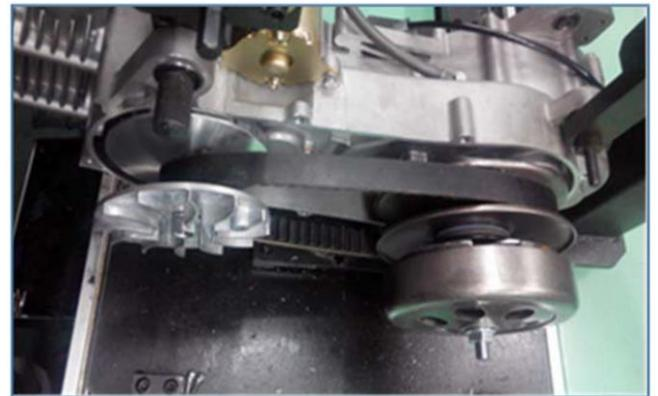
Assemble the clutch that has been installed in the drive belt on the drive axle.
