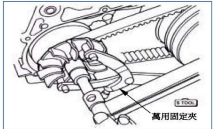
Remove the drive belt from the belt pulley.
