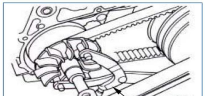
that the belt is separated from the drive plate shaft hub.
