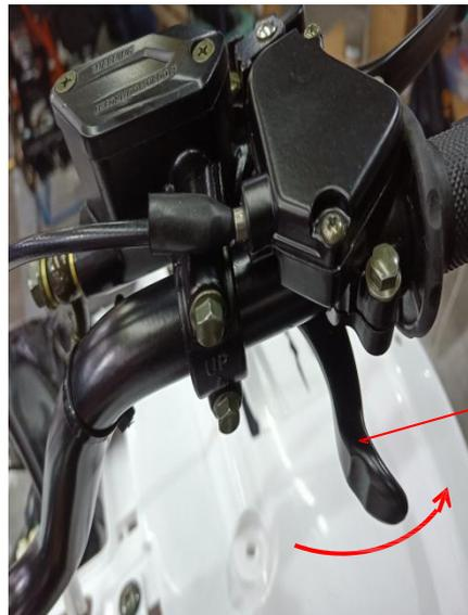
Check the free stroke of throttle button 1
