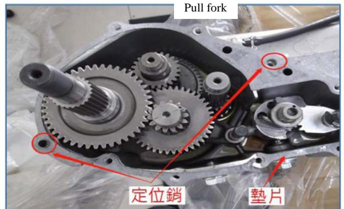
Install positioning pins (2) and new gaskets.
