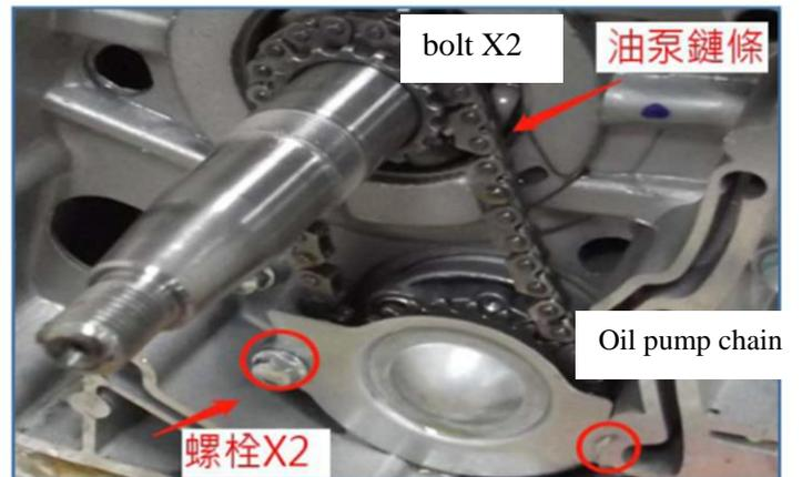
Install the oil pump chain and lock the oil pump cover (bolt X2)
