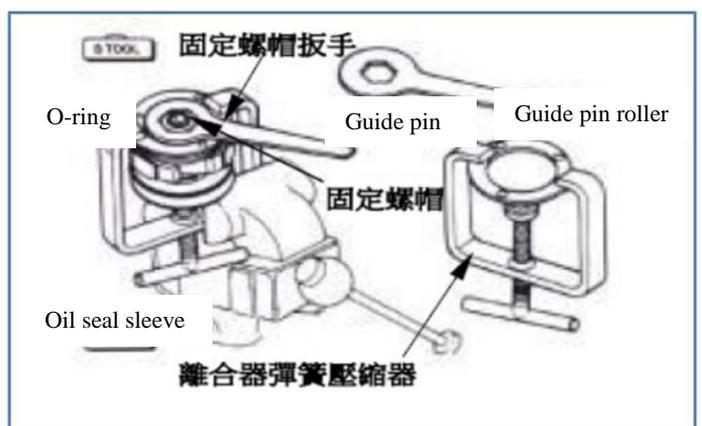
Install the drive belt disc, spring and clutch into the clutch spring compressor, and turn the compressor handle to press down the assembly until the fixed nut can be installed.
