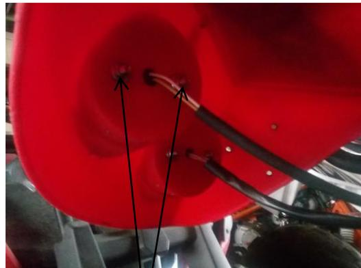
Disconnect the ignition switch lock connector 2
