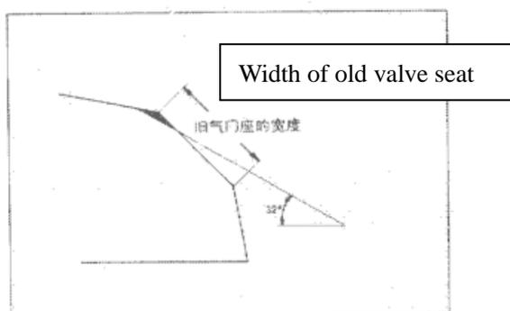
Apply ink to the valve seat and insert it into the valve to rotate
