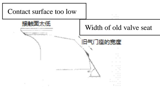
After the valve seat is finished, the valve seat should be coated with abrasive. Then, install the valve and grind the upper valve with a rubber head for grinding. After grinding completed, clean all abrasives remaining on the cylinder head, valve seat and valve guide.
