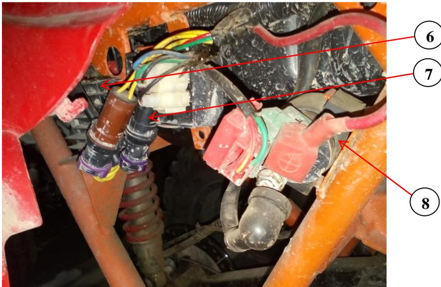
6、 Voltage regulator rectifier 7, charging connector 8, relay
