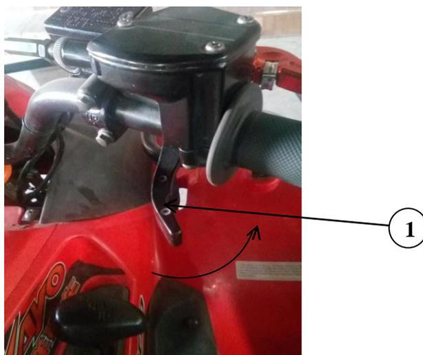
Adjust the clearance when the clearance is not within the specified range
