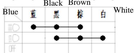
Stop switch / Electric starter switch wiring diagram
