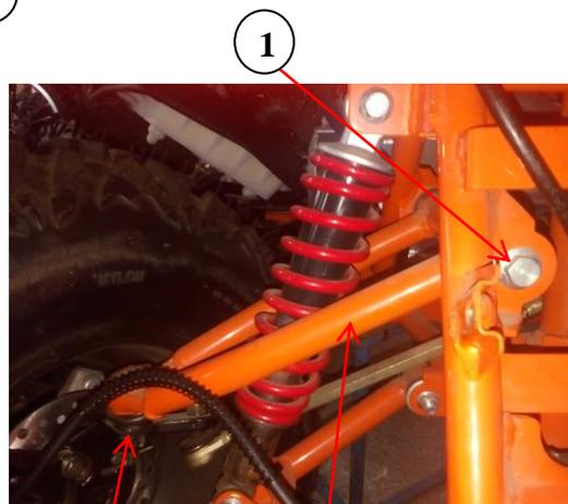
Remove the bolts and nuts that are attached to the frame by the right front lower rocker arm. 5
