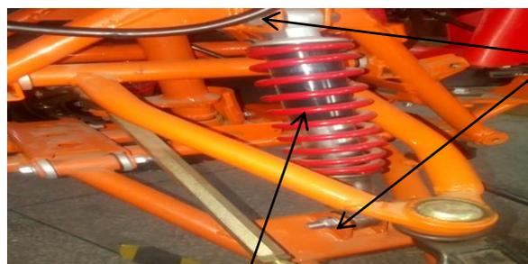
Remove the bolts on the frame and the nuts that fasten the bolt 7 on the right front upper rocker arm 1
