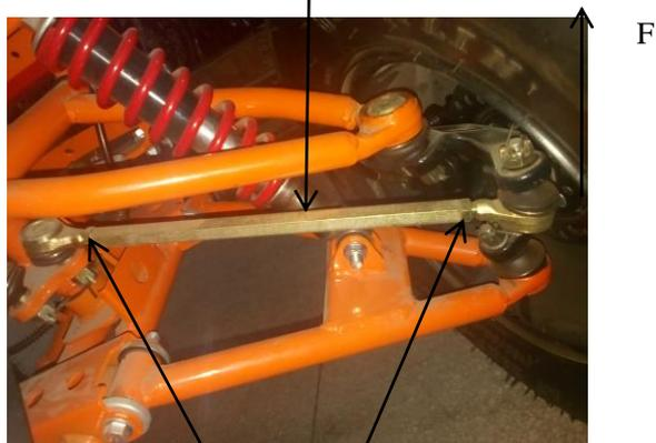
If not in this range, adjust the lock nut<sup>2</sup> of the steering rod 1
