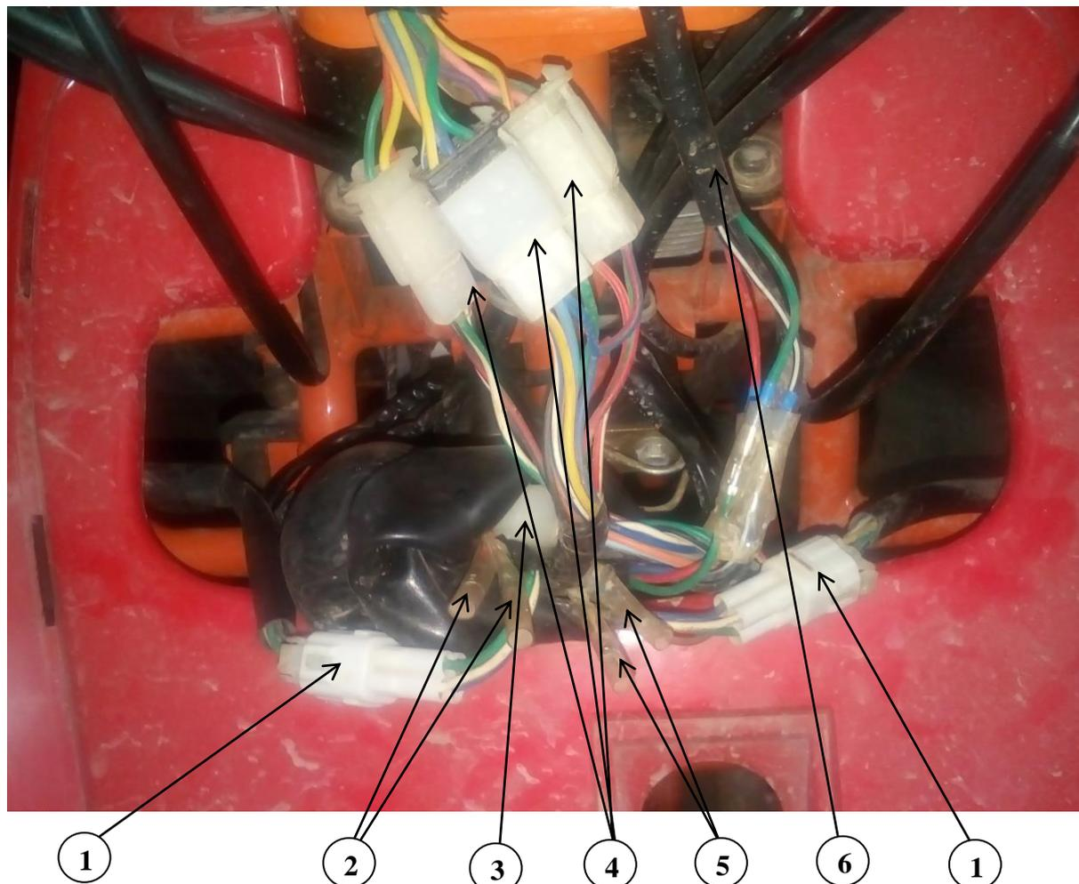
1. Headlight connector 2. Left turn signal connector 3. Left hand multi-function switch connector 4. Instrument connector 5, right turn signal connector 6, electric door lock switch connector
