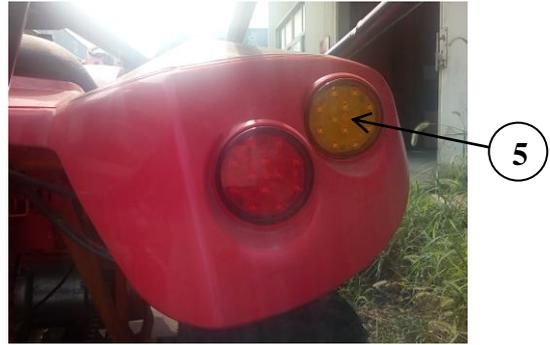
Disassemble the rear taillight socket
