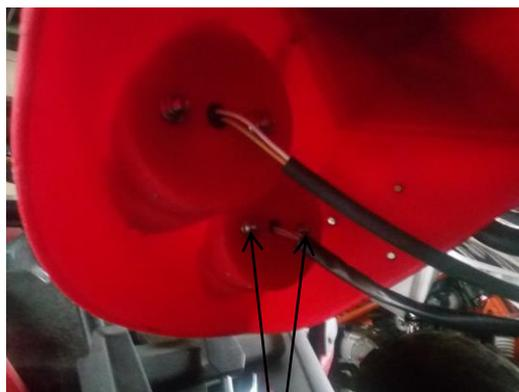
Disconnect the front turn signal connector 2
