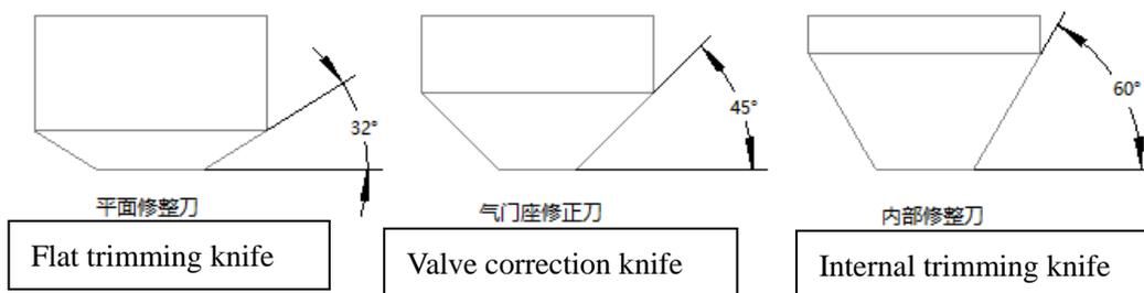
Milling the upper ring of the valve seat with a 32° milling cutter
