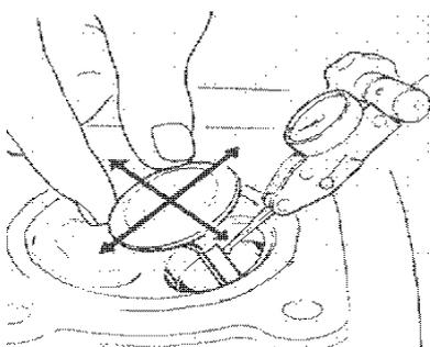
Measuring the free height of the inner and outer springs of the valve
