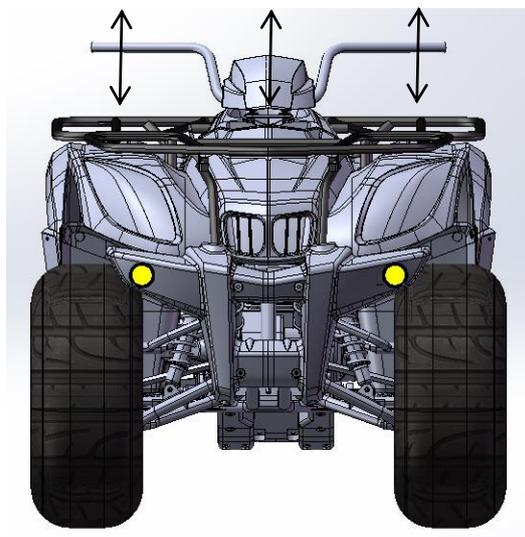
Place the car in a horizontal position and slowly turn it to the left and right to confirm whether it can be rotated smoothly and flexibly. If there is any obstruction in some places, check the main cable assembly and the cable type for interference. If the position of the end of the steering rod is not observed, check for interference and whether the steering bearing is damaged.
