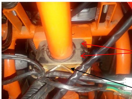
Remove the bolts on which the rear shock absorber is mounted on the car body and on the flat fork assembly 1
