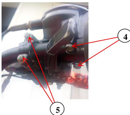
Disassembly of the left hand switch
