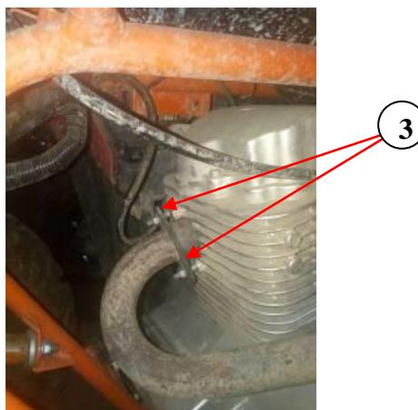
Remove the muffler barrel mounting bolt 4
