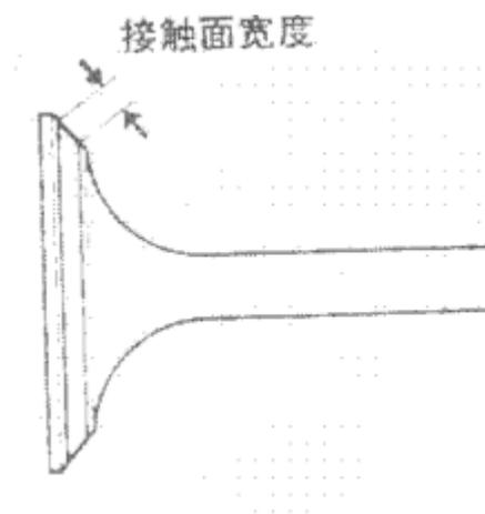
Measuring the width of the valve seat contact surface
