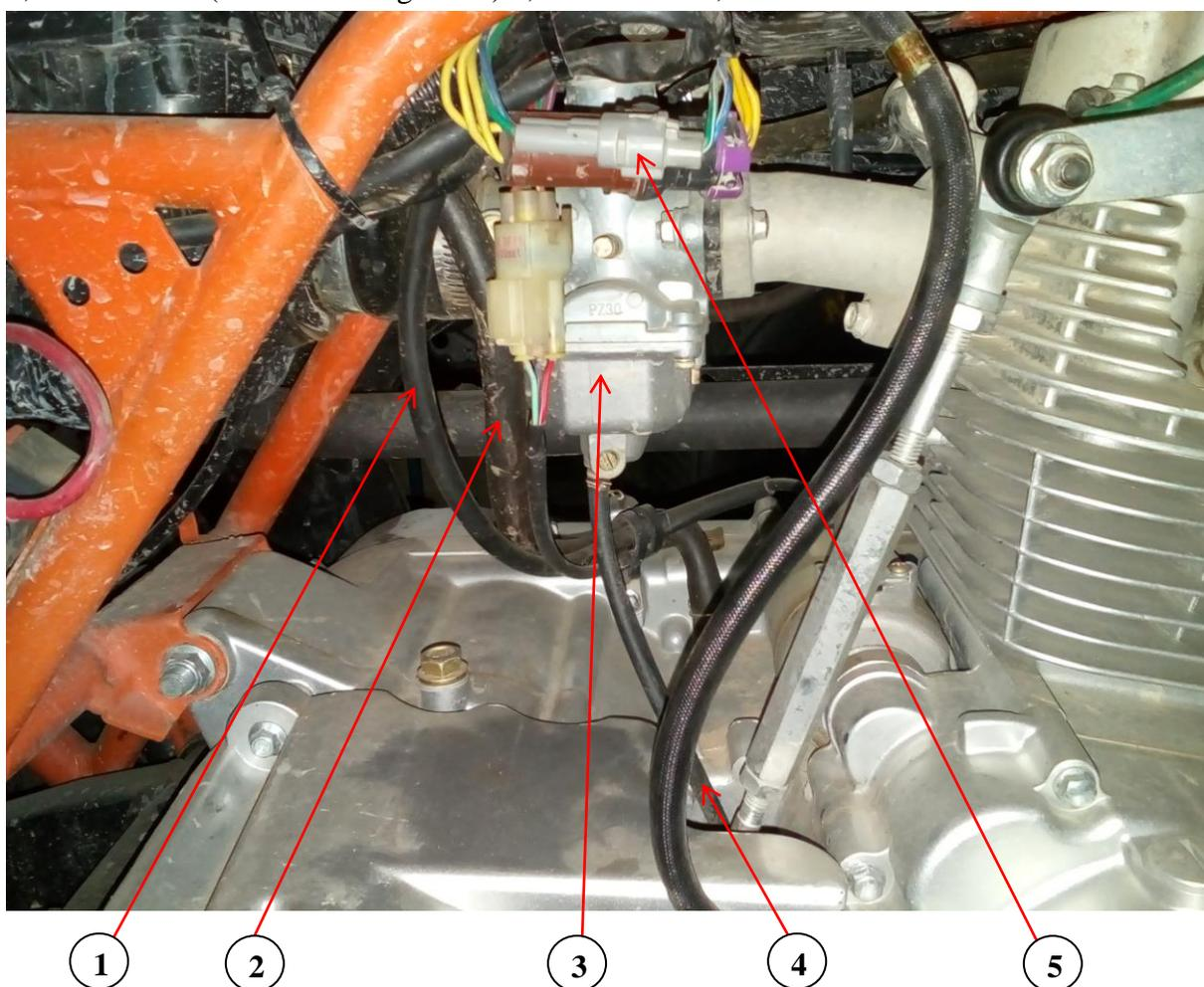
1. Motor line 2. Crankcase exhaust pipe 3. Carburetor 4. Carburetor drain pipe 5. Magnetic motor trigger connector
