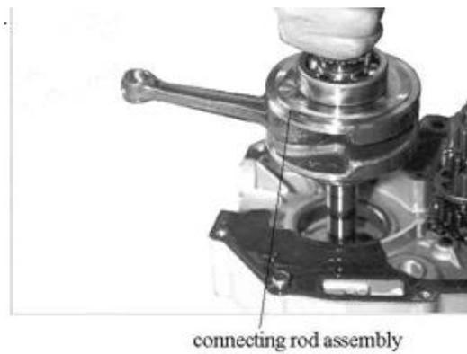
Inspect connecting rod bearing for wear and damage. Replace if necessary.
