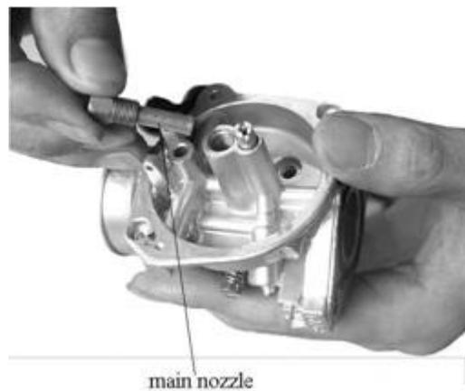
Remove the idle jet and check for plugged. Clean the jet with compressed air if necessary
