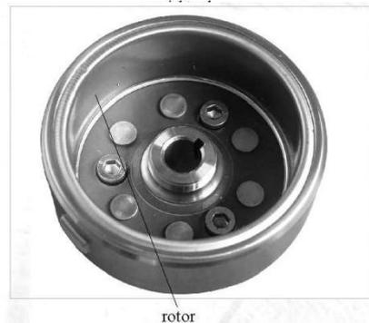
Dis-assemble over running clutch fixing bolt.
