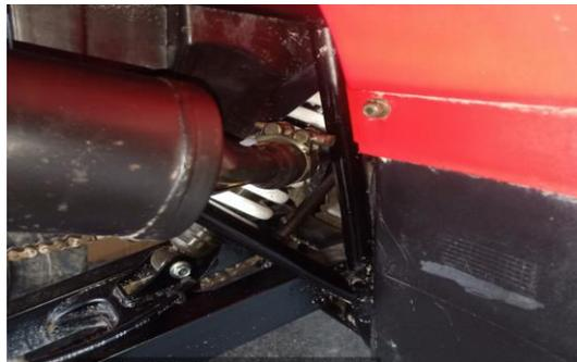
Remove the washer of muffler to inspect for damage. Replace if necessary.
