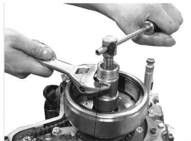
Check if rotor is with magneto. Change if necessary.
