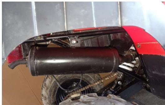
Remove the muffler to inspect for broken and damage. Replace or repair if necessary.
