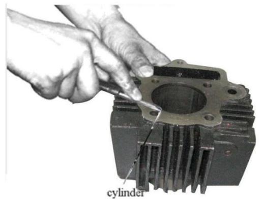
Check the state of cylinder inner wall .Replace if worn or if reuse is questionable.
